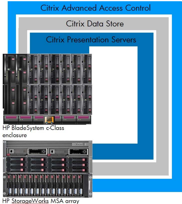
Figure 6: A typical server farm, with storage for the data store deployed on an HP StorageWorks MSA1500 array
